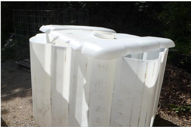
Lower IBC: In order to have a bucket within a bucket, cut the top of one IBC right below the curve.
