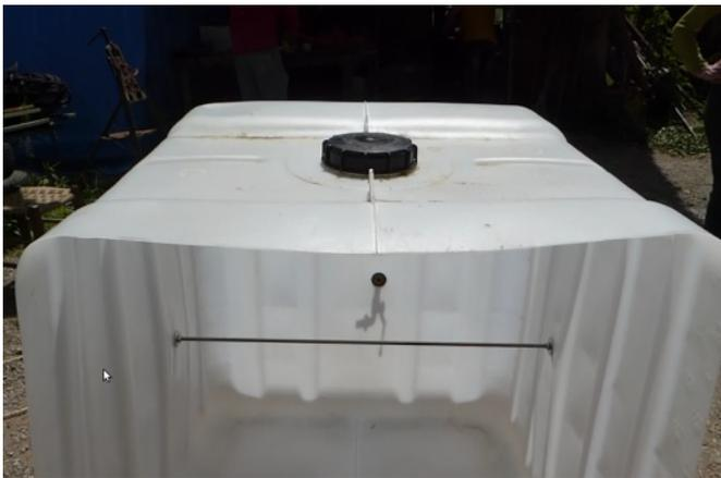
To stabilize the floating drum add a stainless steel threaded bar with two nuts, washer and rubber ring on each side. Make the bar a bit shorter, that the tank is pulled together (2").
